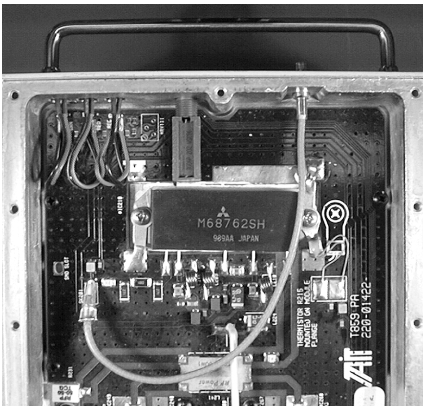
Figure 3.4 T859 Front RF Input Coax Routing
